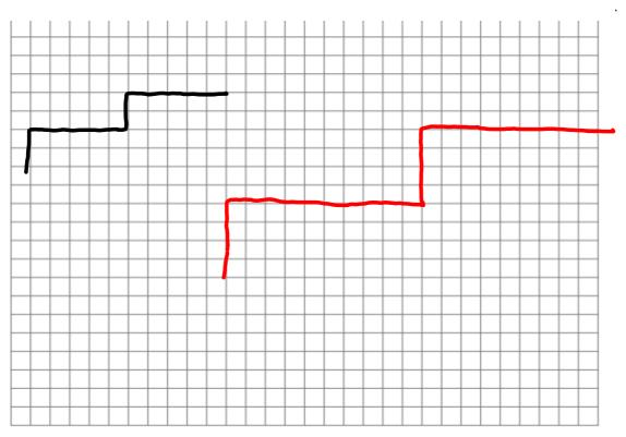
2. Each step of the staircase is to have a 12" tread. Accurately draw this on the graph paper (scale: 1 unit = 1 inch). What is the vertical rise of each step of a 12" tread, for a slope of <sup>2</sup>/<sub>5</sub>?
